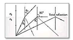
When the angle of incidence is greater than the critical angle, the incident ray is reflected back to the medium. We call this phenomenon as total internal reflection. An application of this phenomenon is found in optical fibres.
